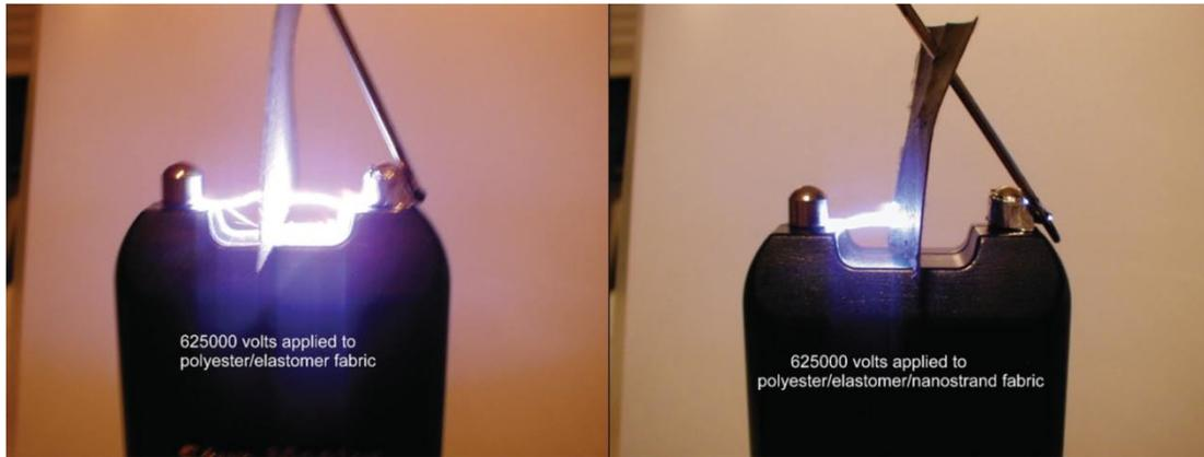
**Figure 7.** A 625,000 volt discharge readily passes through a non-conductive composite at the left. But with the addition of 5% volume nanostrands to the resin, the same discharge is effectively controlled [13]
