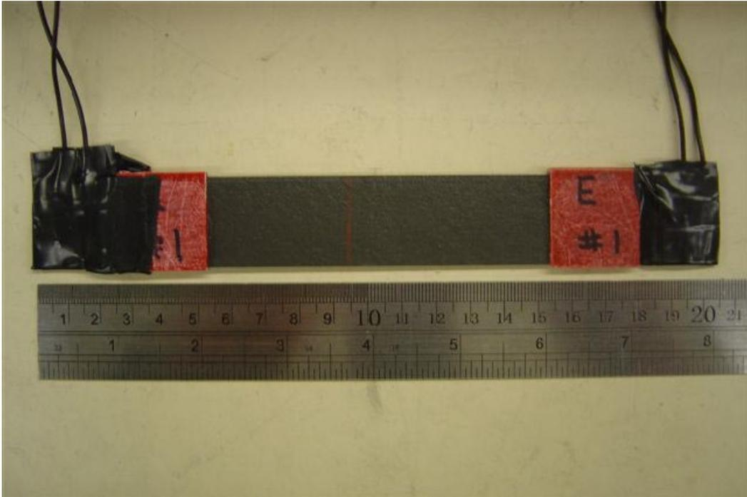
**Figure 11.** M55J/RS-3 with exterior nickel nanostrands<sup>TM</sup> tensile specimen.
