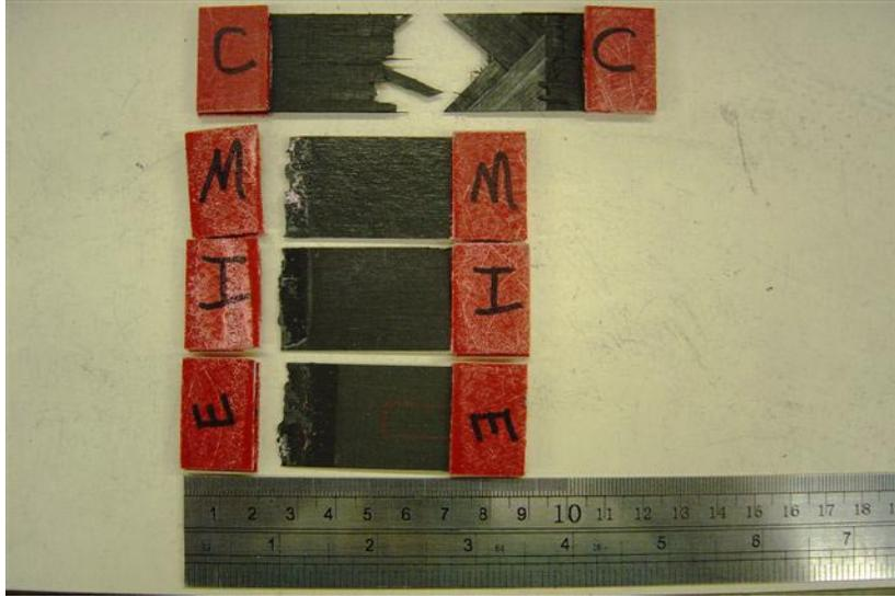
**Figure 72.** Fracture of 7.62 cm Irradiated Specimens
