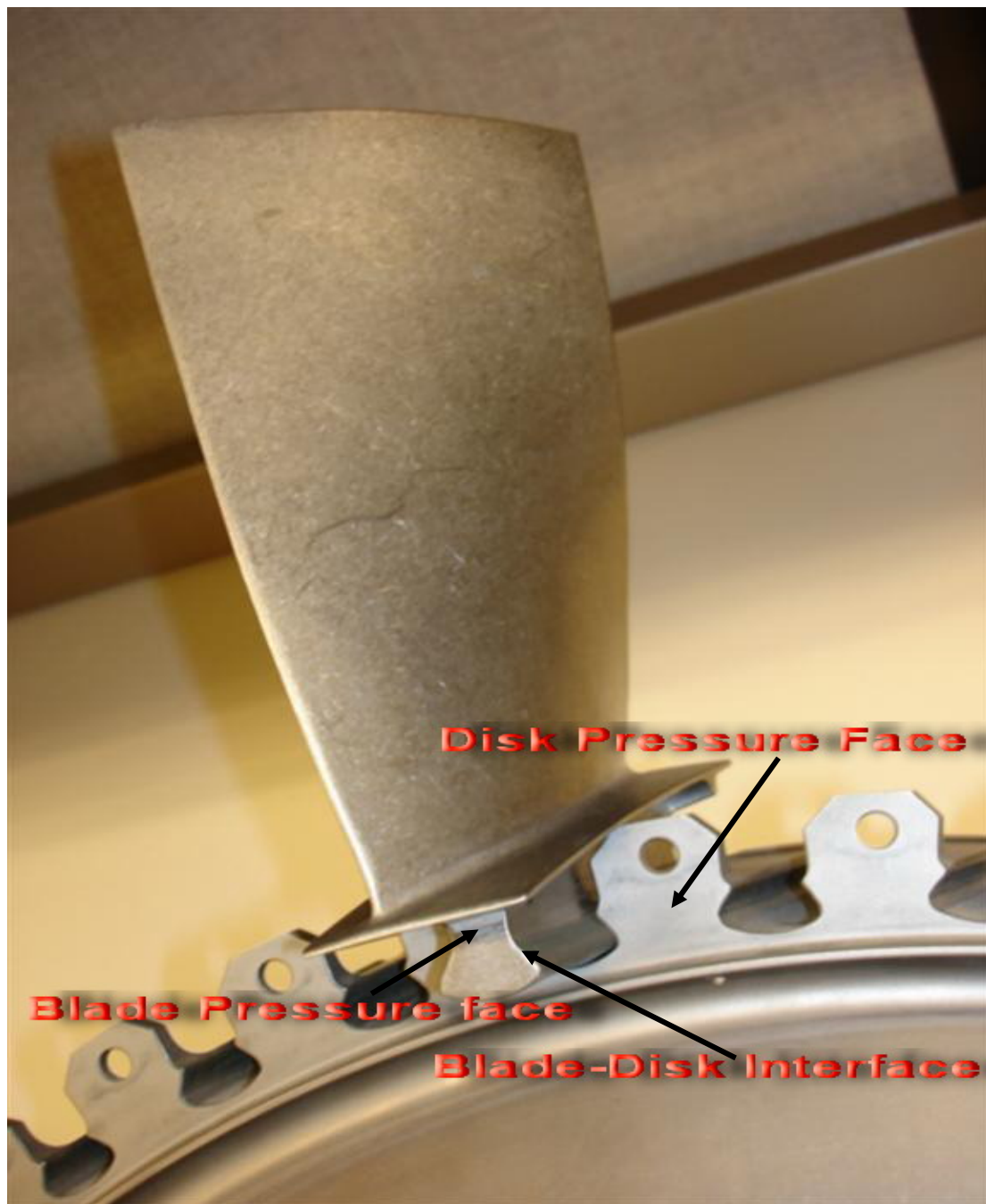
Figure 1.1 Blade/Disk Dovetail Joint in a Turbine Engine
