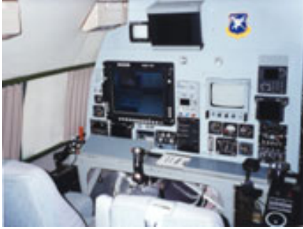
Figure 23 – View of Aft Crew Compartment inside TIFS
