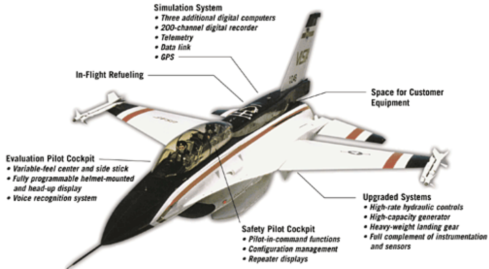
Figure 26 – Capabilities of the Variable-Stability In-Flight Simulator Test Aircraft
