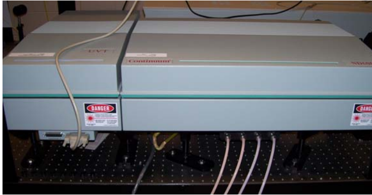
Fig. 2. ND6000 narrowband dye laser with frequency doubler
