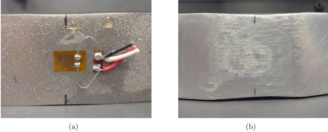
Figure 4.3: Minor Disbonding (a) and Complete Delamination (b) of the Strain Gage and Terminal Pad
