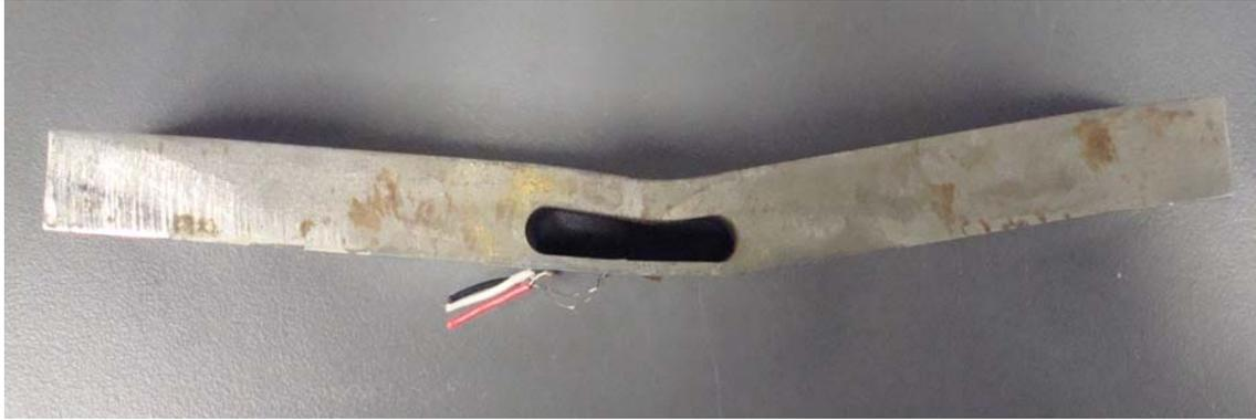
Figure 4.2: Global Deformation of Slotted Beam Specimen Resulting from Off-Center Impact
