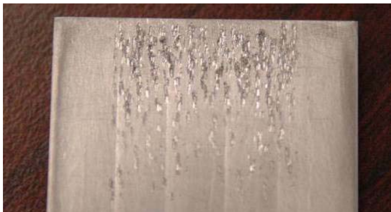
Figure 4.6 Marks on Aluminum Bar Produced by Slipping Grips
