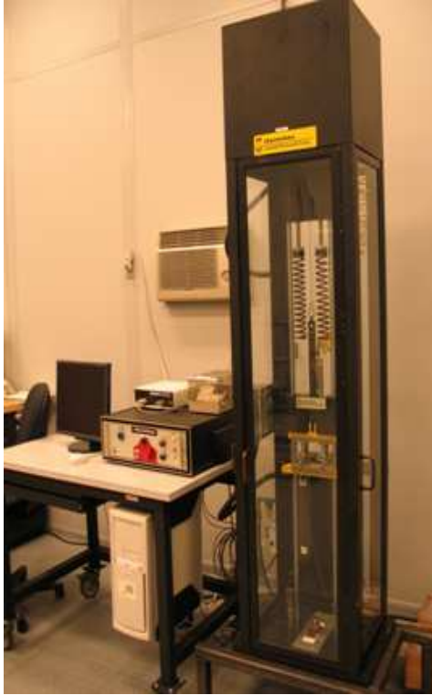
Figure 5.1: Dynatup apparatus used for low- to medium-energy impact testing.
