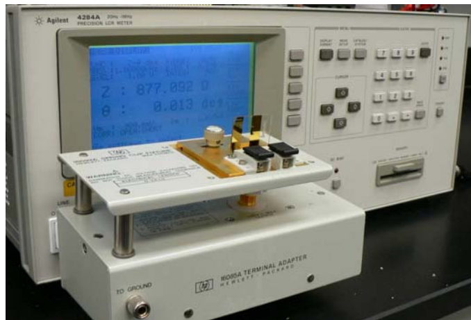
Figure 5-3: Dry-run measurement setup on Agilent 4284A precision LCR meter using Thornell® P-100 fiber suspended between two gold metallized contacts on a glass slide. Note that gold is facing LCR meter screen to make contact with metal electrodes on the terminal adapter [53].
