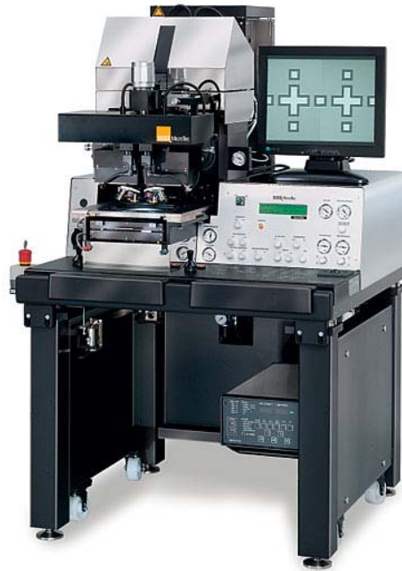
Figure 6-4: Karl Süss MA-6 mask aligner used to pattern 3350 photoresist on PolyMUMPs ® die.
