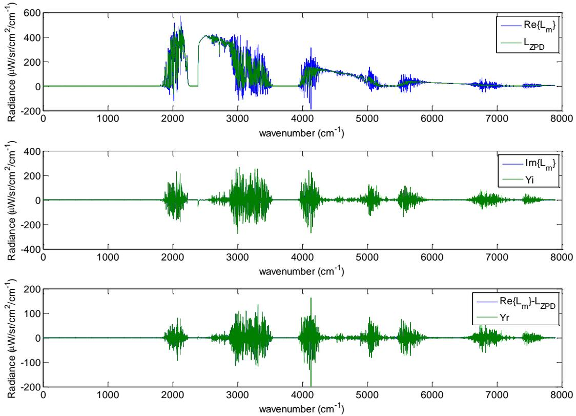
**Figure 6. FTS spectrum of black body with atmospheric transmission path length of .5 km and a temperature change from 1500 K to 600 K during data acquisition.**
