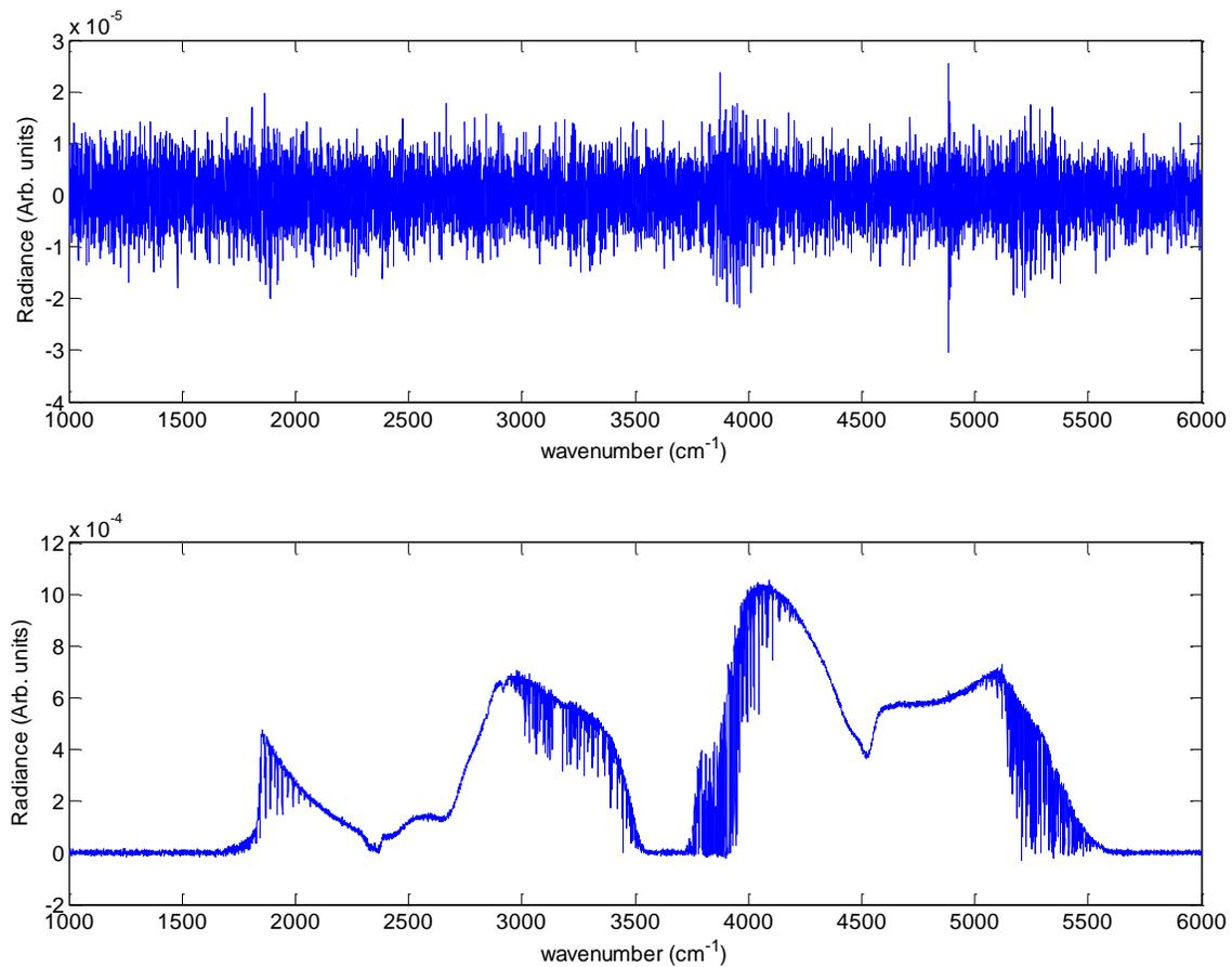
**Figure 18. Measurement 10 spectrum at 17.14 seconds with a ZPD voltage = 1.481 V, imaginary on top and real on bottom, of a decaying incandescent lamp. Measurement time corresponds to a few SCA spectral peaks in the imaginary spectrum.**
