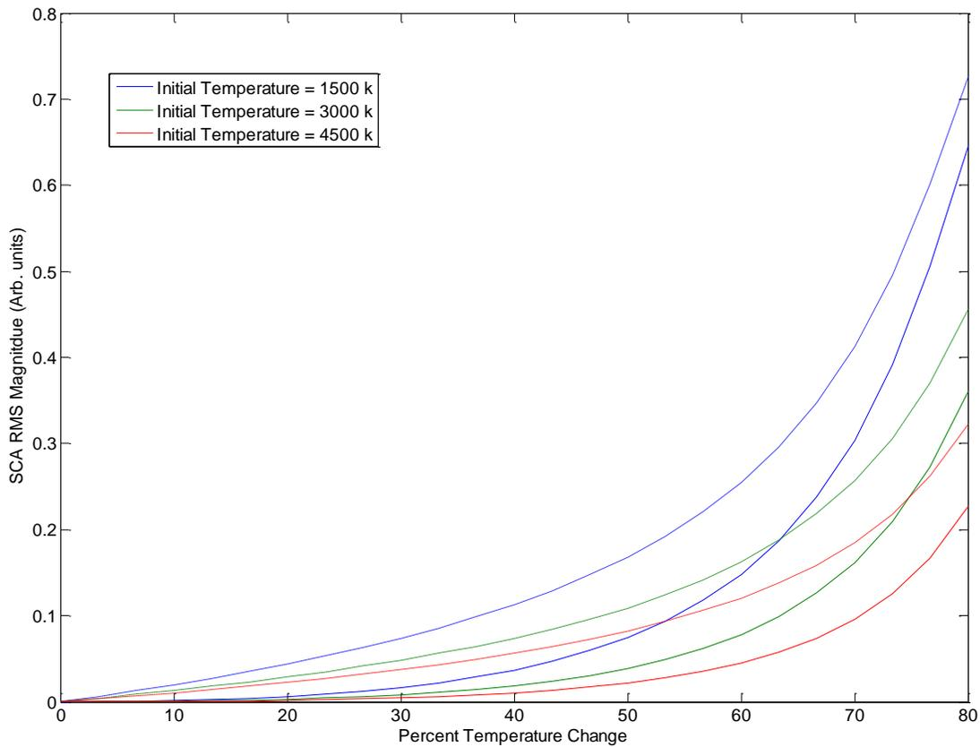
**Figure 11. The three scenarios correspond to different initial temperatures of 1500 k, 3000 k, and 4500 K. Dashed lines represent the  $\text{SCA}_{\text{Im}}$  while the solid lines represent the  $\text{SCA}_{\text{Re}}$ . MOPD = .5 cm and Atmospheric transmission path length = .5 km.**
