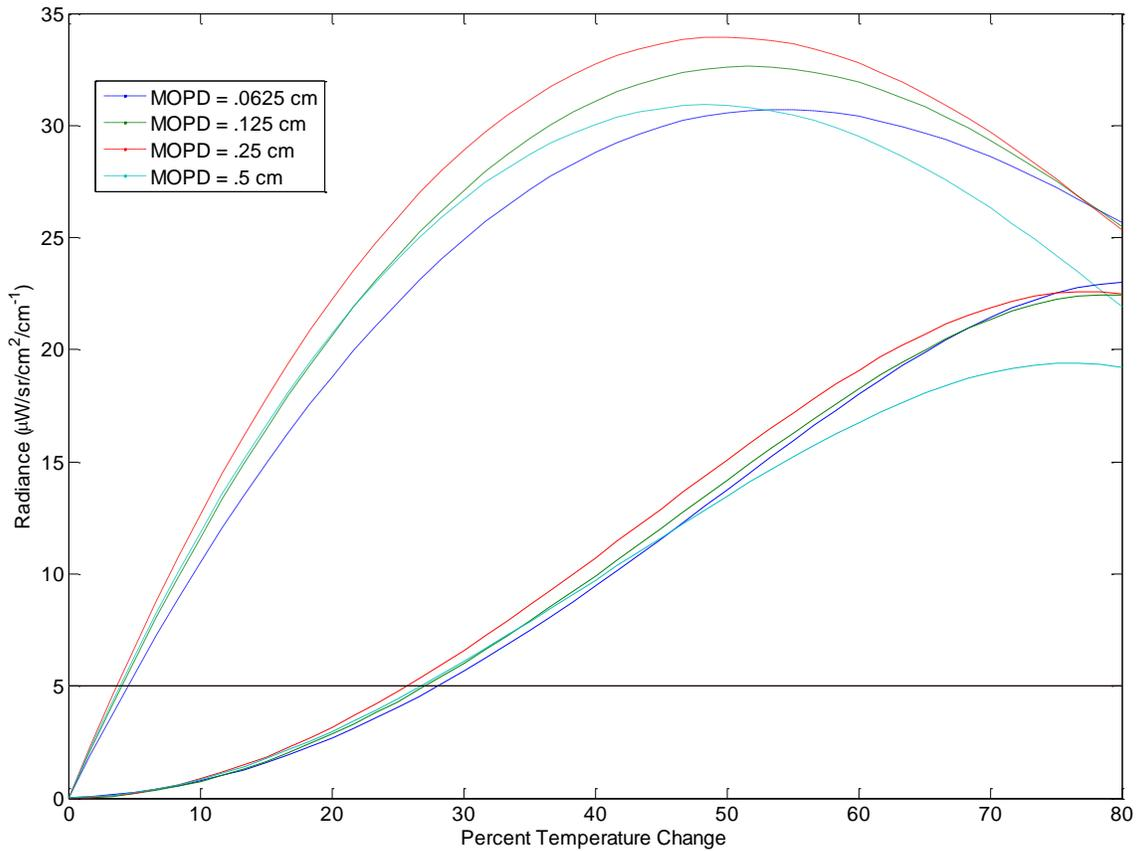
**Figure 15. RMS of  $\text{Im}\{L_m\}$  (dashed) and the RMS of  $\text{Re}\{L_m\} - L_{ZPD}$  (solid) values as they change with temperature change. The black horizontal line represents a NESR of  $5 \mu\text{W} / \text{sr} / \text{cm}^2 / \text{cm}^{-1}$  that both  $\text{Im}\{L_m\}$  and  $\text{Re}\{L_m\} - L_{ZPD}$  must rise above for SCAs to be distinguishable.**
