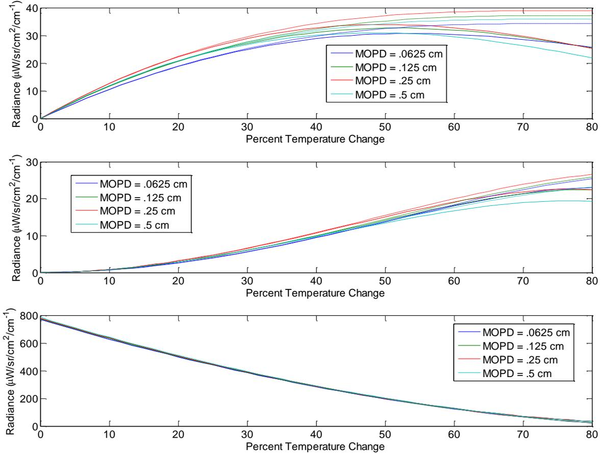
**Figure 14. Dashed lines represent theoretical predictions based on implementing Equation (21) based on Kick et al. The solid line represents the actual modeled values. Top) Deviation of RMS values of  $\text{Im}\{L_m\}$  and  $Y_i$ . Middle) Deviation of the RMS of  $\text{Re}\{L_m\} - L_{ZPD}$  and  $Y_r$ . Bottom) Deviation of the RMS of  $\text{Re}\{L_m\}$  from the RMS of  $L_{ZPD}$ .**
