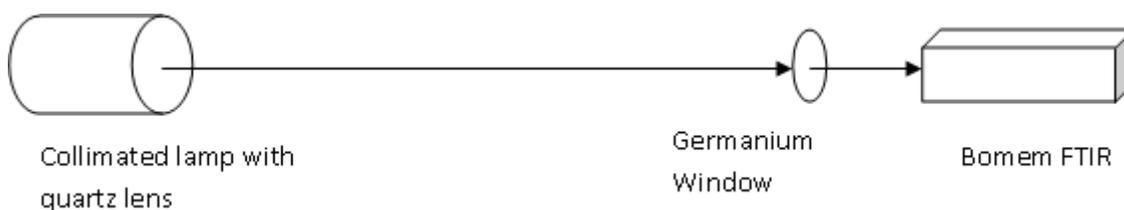
**Figure 16. Experimental Setup**
