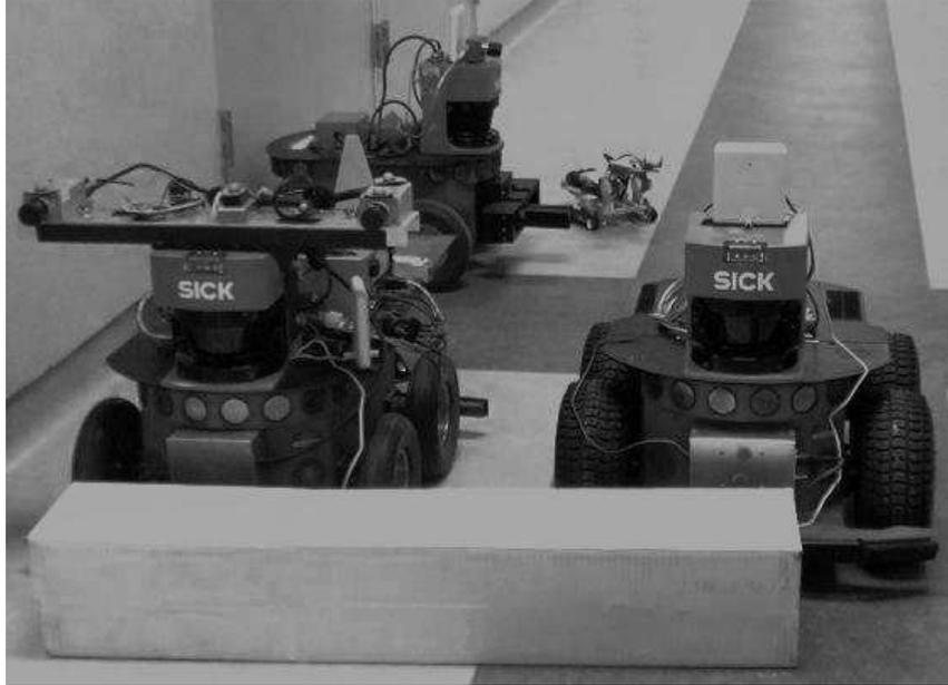
Figure 6.1: The robotic collective executing the MOVE\_ITEM task. The two robots in the foreground are Frodo and Gandalf, the robots in the background are Gollum and the NXT.
