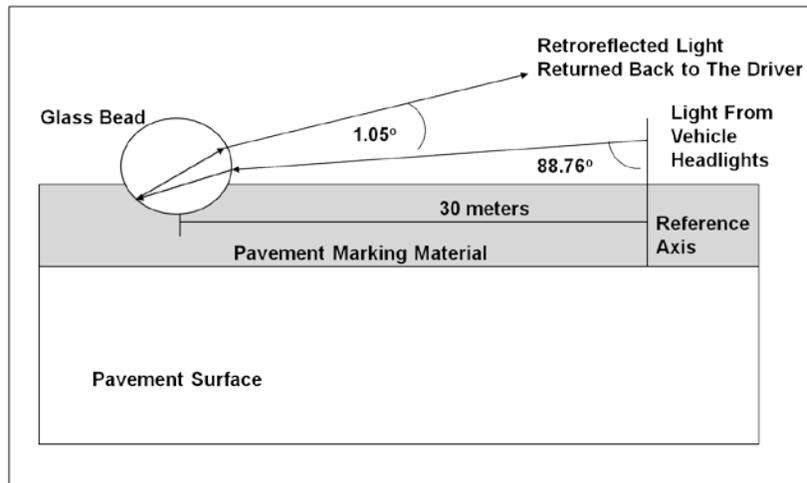
**Figure 1. Glass bead retroreflectivity physics (Rasdorf et al. 2009).**
