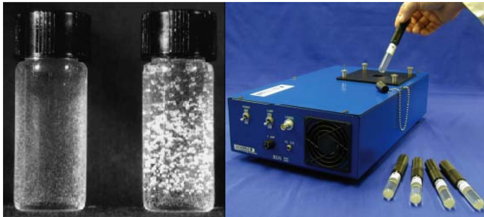
Figure 6. Left: The SDD is a vial of gelatinous liquid containing superheated drops that neutrons interact with, causing voids that can be counted. Right: The SDD reader is an easy way to count the voids created by neutrons in a superheated drop detector.
