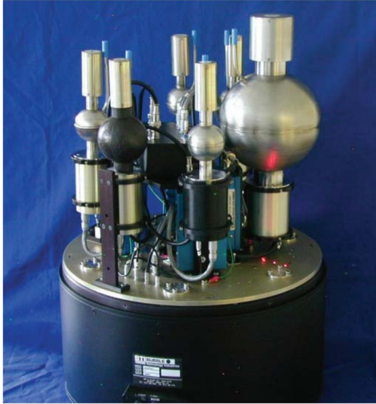
Figure 5. The ROSPEC is a completely self-contained neutron spectrometry system capable of measuring neutron energies from thermal through fast.
