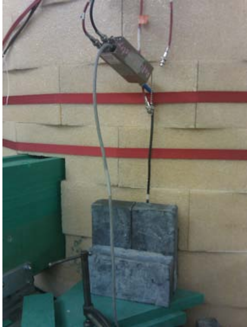
Figure 24. The outer shell of the NREP TMR is made from blocks of borated materials used to absorb neutrons and limit the radiation exposure to equipment located outside the TMR cylinder.
