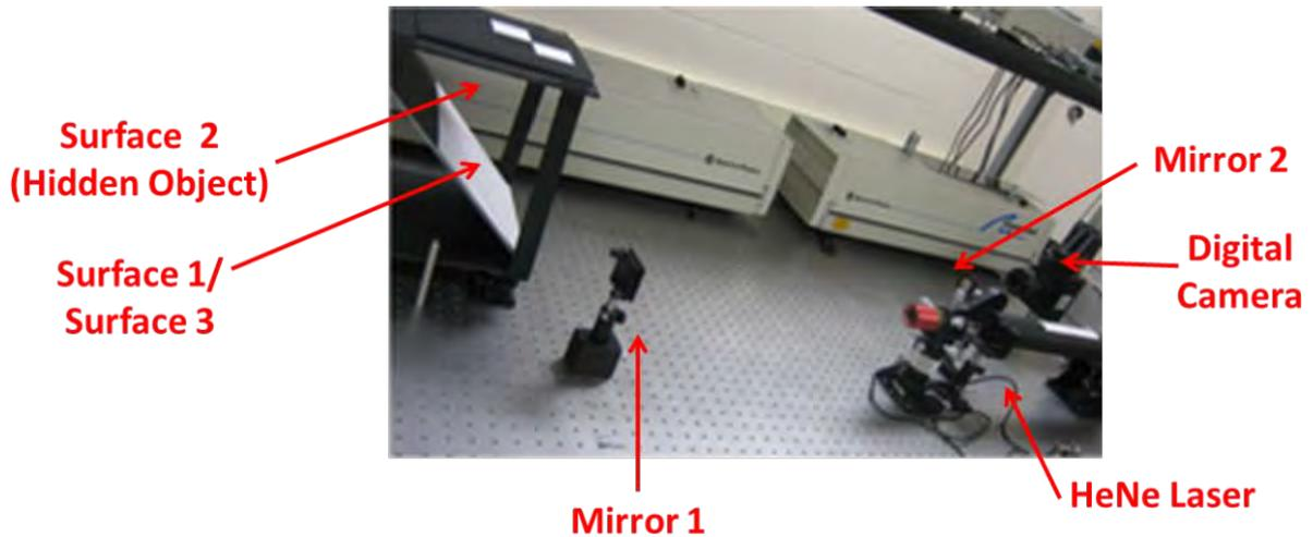
Figure 5. Prior experimental setup (Ferrel, Schafer, & Powell, 2011).
