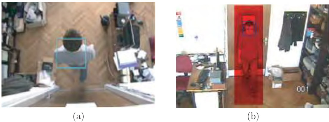
Figure 2.2: Example of two part system developed by Draganjac et al. [1]. The first camera in (a) allows the detection and tracking of a dismount. The second camera in (b) searches for a face to see if it is concealed or not.
