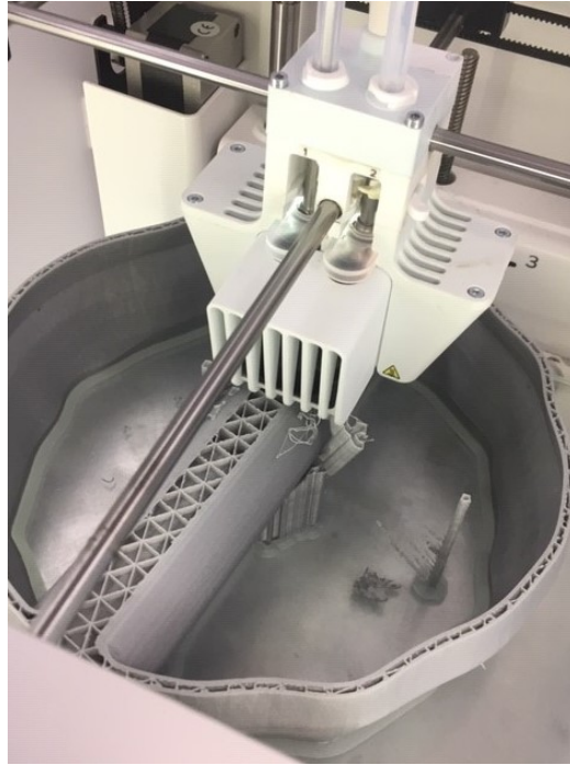
Figure 7: Printing bottom of model in Ultimaker 3
