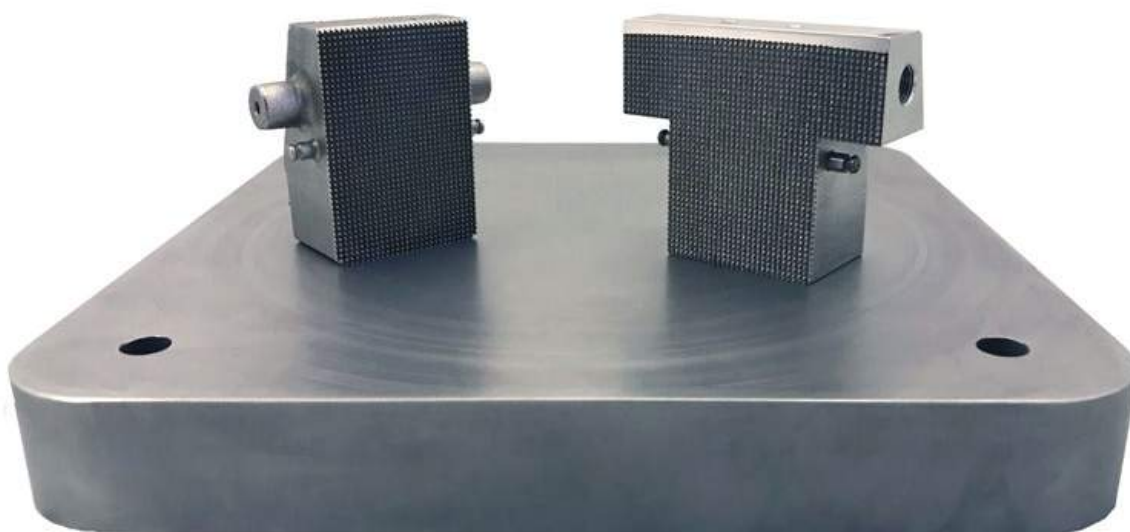
Fig. 3 Initial AM design (left) with 3.0 mm diameter triple loop interior channel; final AM design (right) with 5.0 mm diameter single loop interior channel
