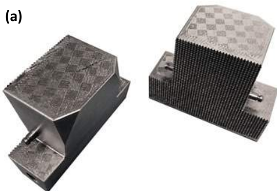
Fig. 7 (a) shows the finished printed parts with the island scan strategy shown as a checkered pattern. Part orientation in Magics build scene on the M2 platform is shown in (b). The red circles on the platform indicate build plate screw hole locations
