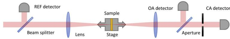
**Fig. 1.** Z-scan technique. The sample is scanned through the focus of a Gaussian beam. The open aperture (OA) detector measures the total power transmitted and is sensitive to the nonlinear absorption (NLA). The aperture before the closed aperture (CA) detector makes the detector sensitive to the self-focusing/defocusing of the beam and hence the nonlinear refraction (NLR). A reference detector is used to account for laser power fluctuations.
