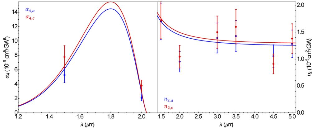
**Fig. 3.** Measured values of  $\alpha_4$  compared for  $a$ -axis (blue) and the  $c$ -axis (red) compared to the Wherret model. Right) Measured values of  $n_2$  for  $a$ -axis and the  $c$ -axis compared to the two band Kane model.
