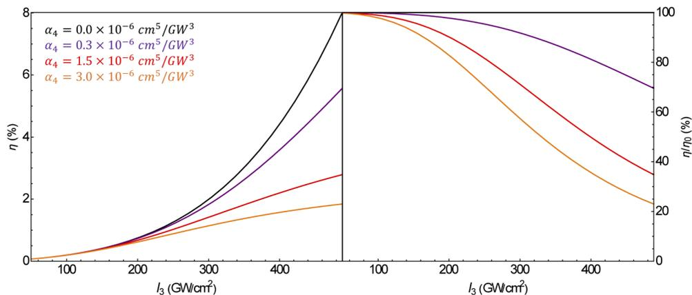
**Fig. 6.** (Left) Conversion efficiency for the case of a 3.3  $\mu\text{m}$  signal, 2.0  $\mu\text{m}$  pump and 5.0  $\mu\text{m}$  idler vs. pump irradiance for a  $L=100 \mu\text{m}$  crystal with and without 4PA for various values of  $\alpha_4$ . (Right) Normalized conversion efficiency  $\eta/\eta_0$  for various values of  $\alpha_4$
