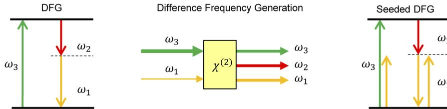
**Fig. 4.** Left) Difference frequency generation. The pump  $\omega_3$  is broken into two photons of lower energy, the signal  $\omega_1$  and the idler  $\omega_2$ . (Center) and (Right) In our model we seed the interaction with a seed to stimulate the production of the idler.
