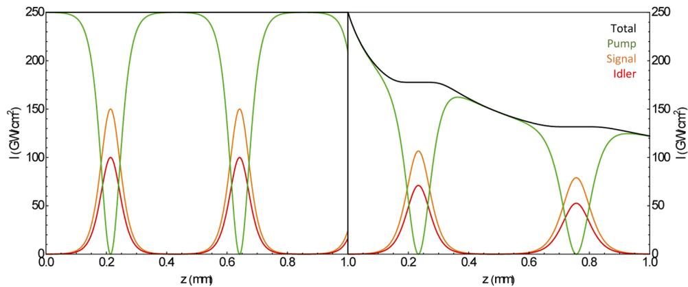
**Fig. 5.** (Left) Irradiance of the 3.3  $\mu\text{m}$  signal (orange), 2.0  $\mu\text{m}$  pump (green) and 5.0  $\mu\text{m}$  idler (red) beams propagating in the crystal in absence of 4PA. The pump is set to  $I_3 = 250 \text{ GW/cm}^2$ . The energy is continuously exchanged between the beams. (Right) In the presence of 4PA ( $\alpha_4 = 3.0 \times 10^{-6} \text{ cm}^5/\text{GW}^3$ ) the signal and idler are reduced as the pump is attenuated.
