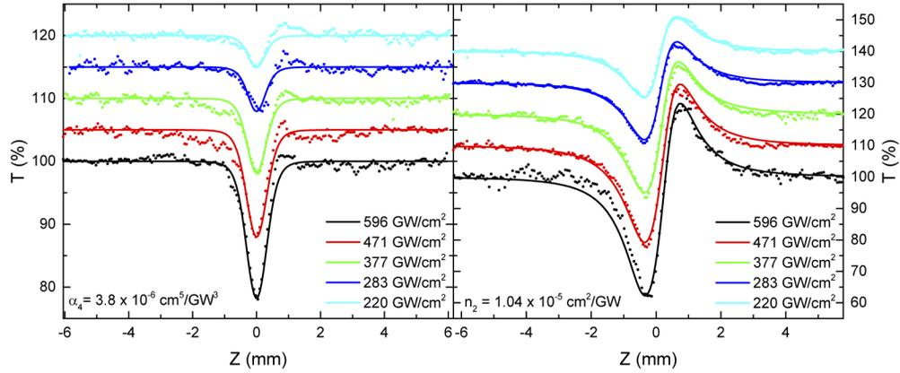
**Fig. 2.** Z-scans of CSP at  $2.0 \mu\text{m}$  along the  $c$ -axis at various peak irradiances. Signals show normalized transmission  $T$  vs. sample position  $Z$  relative to beam focal position. Left: OA signal and fit with  $\alpha_4$ . Right: CA signal with fit for  $\alpha_4$  and  $n_2$ . Plots have been shifted vertically for clarity.
