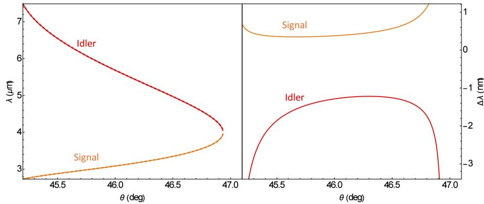
**Fig. 7.** Left) phase matching curves for signal (red) and idler (orange) at low ( $0 \text{ GW/cm}^2$ , solid) and high ( $500 \text{ GW/cm}^2$  dashed) irradiance. The curves lie on top of each other indicating a small difference in output wavelength. Right) Difference between low and high irradiance phase matching curves
