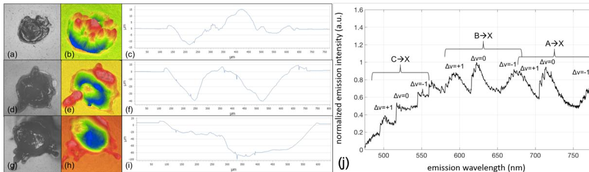
**Figure 1.** Single  $250 \text{ J/cm}^2$ ,  $60 \mu\text{s}$  pulse on Ti wafer optical image (a), white light interferometric image (b), and depth profile (c). Two pulses at 10 Hz repetition rate (d,e,f). Three pulses at 10 Hz repetition rate (g,h,i). Spatially and temporally averaged emission spectra (j).
