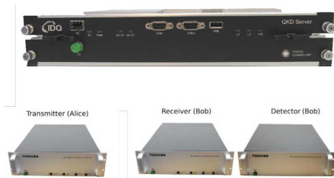
Figure 3. The ID Quantique (IDQ) rack mountable QKD system is shown on the top (ID Quantique, 2016) and the Toshiba record holding hybrid QKD system is shown on the bottom (Dixon, et al., 2015).
