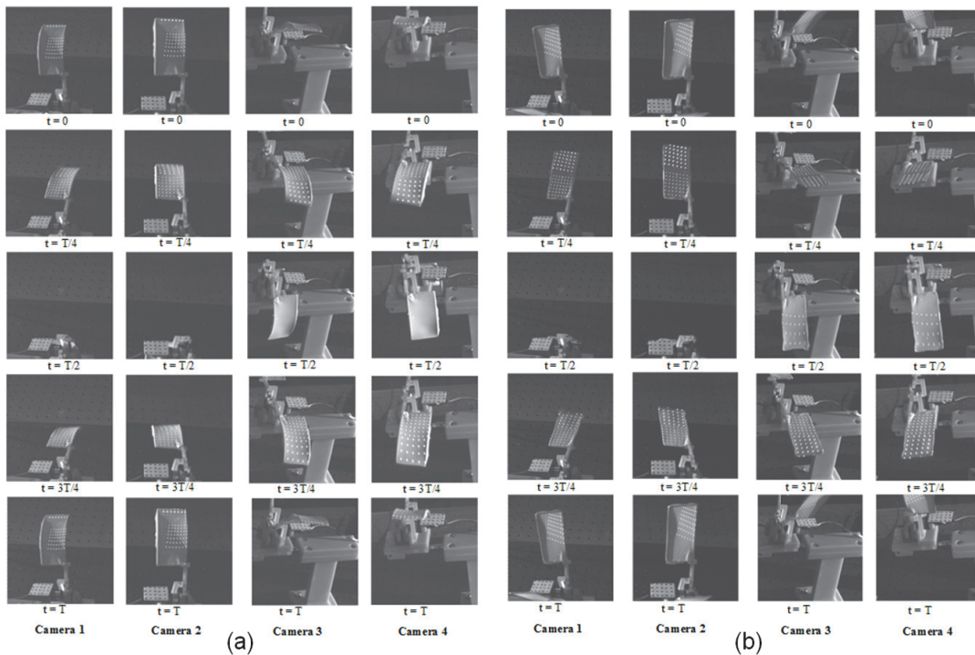
Figure 23. Four high speed camera images of curved (a) and straight (b) tube frame wings with laser dot projection at 6.2 Hz flapping frequency.
