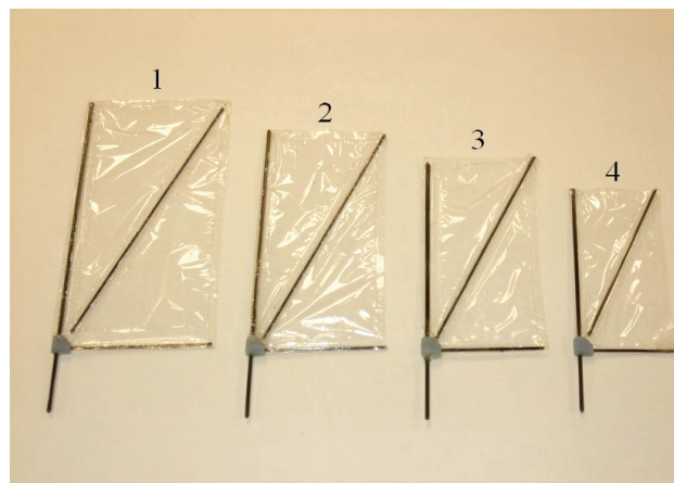
Figure 1. Carbon Fiber Wings with Mylar Membrane. Wing #1 – Spar length = 4" Chord Length = 2" Wing Span = 12.1". Wing #2 – Spar length = 3.5" Chord Length = 1.75" Wing Span = 11.1". Wing #3 – Spar length = 3" Chord Length = 1.5" Wing Span = 10.1". Wing #4 – Spar length = 2.5" Chord Length = 1.25" Wing Span = 9.1".
