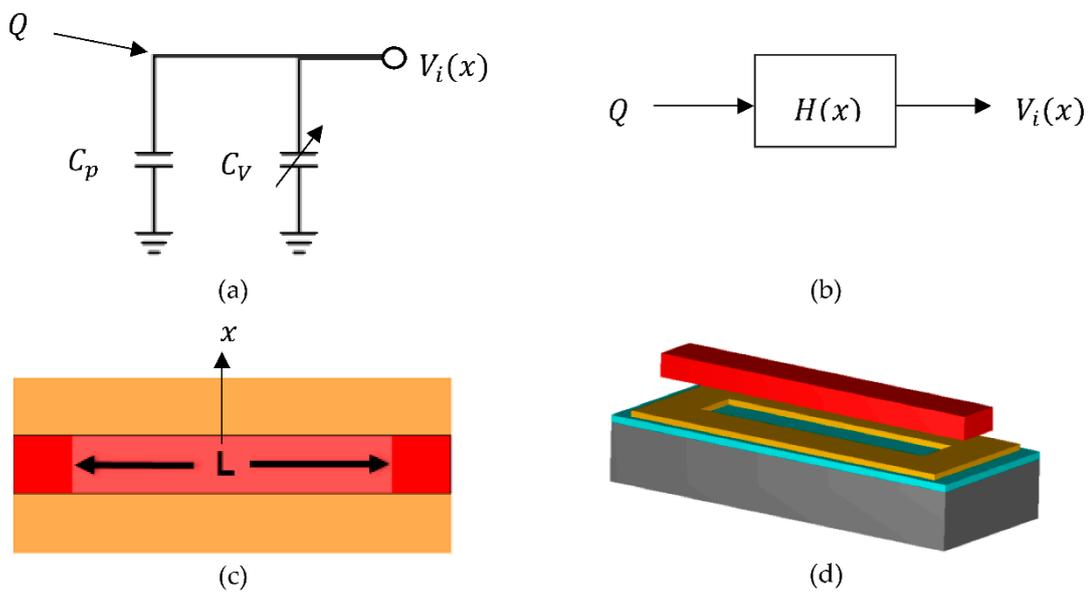
**Figure 1.** This figure shows conceptual pictures of the variable capacitor. (a) shows a simplified circuit where  $C_p$  is the lumped up parasitic capacitances,  $C_v$  is the variable capacitor, and  $Q$  is the charge that induces the sense voltage  $V_i$ ; (b) is a block diagram of the same circuit; (c) is a 2D model of the simple variable capacitor; (d) is a 3D model of (c).
