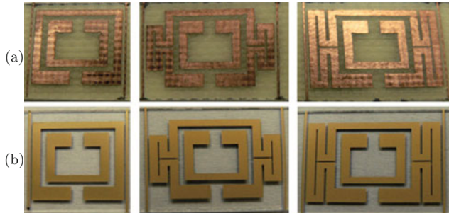
Fig. 2 Baseline, Loop A and Loop B Meta-atom designs, (a) prototypes on printed circuit board and (b) designs made by microelectronic fabrication techniques on quartz substrates.
