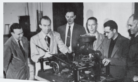
Faculty register various degrees of animation toward a laboratory densitometer, which measures the intensity of spectral lines.
