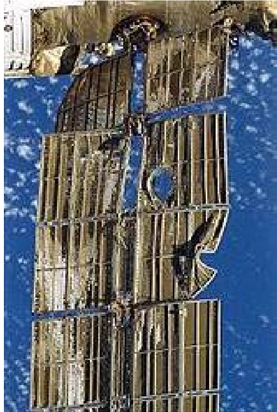
Figure 7. Damage to the Soviet MIR from Docking Accident
