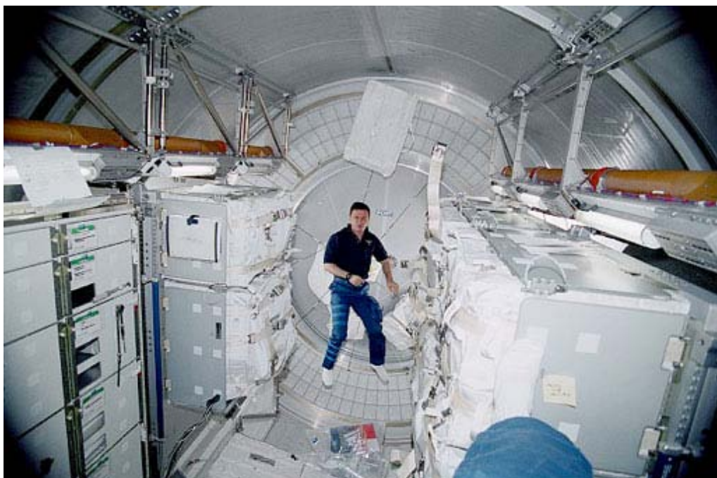
Figure 22. Interior of Italian Multi-Purpose Logistics Modules
