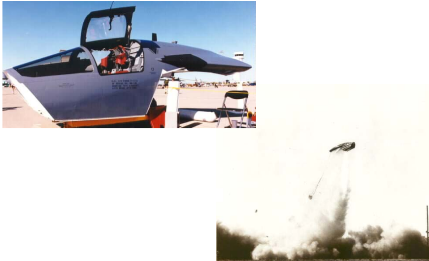
Figure 2-3. Escape Capsule and Test
