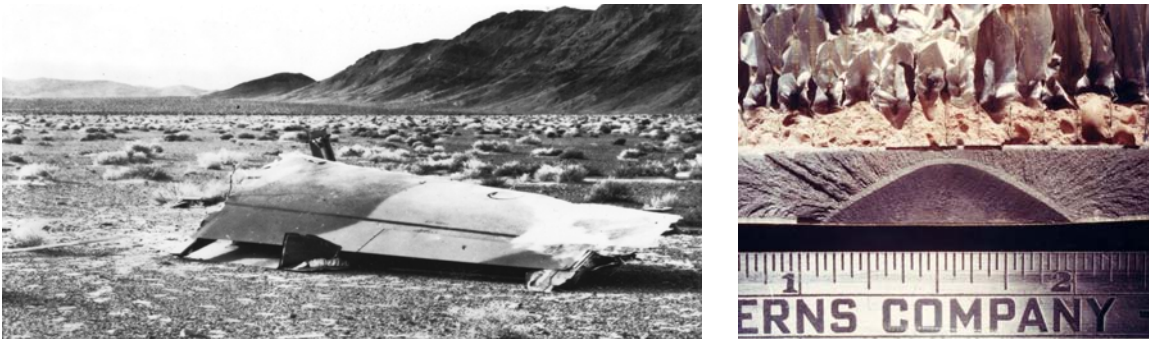
Figure A8-5. Failed F-111 Wing and Forging Defect in Wing Pivot Fitting Lower Plate
