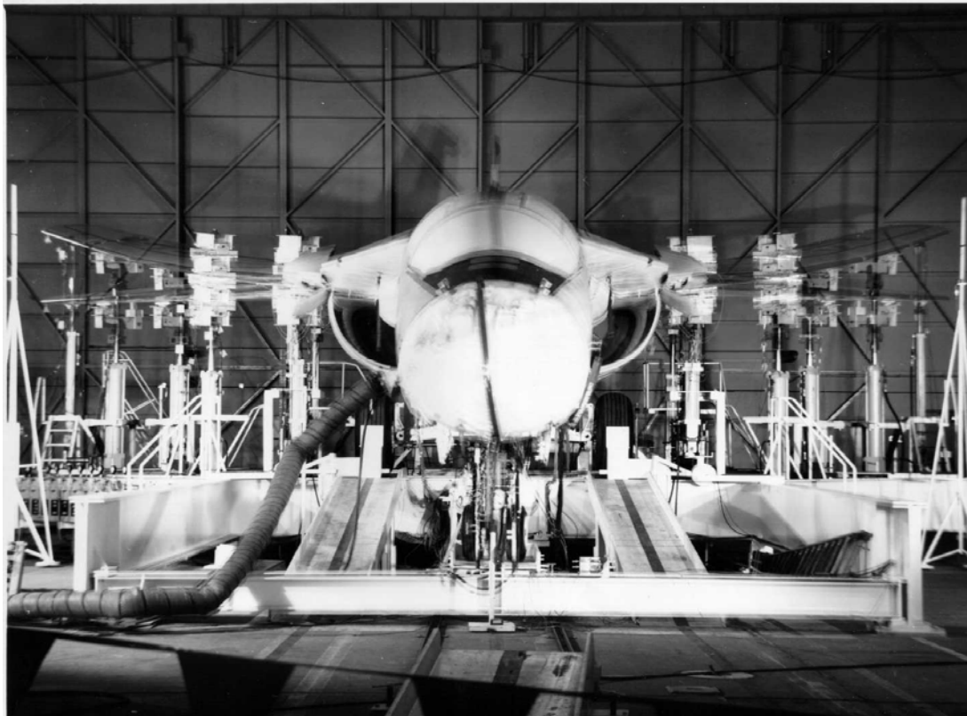
Figure 3-11. F-111 Cold Proof Load Test
