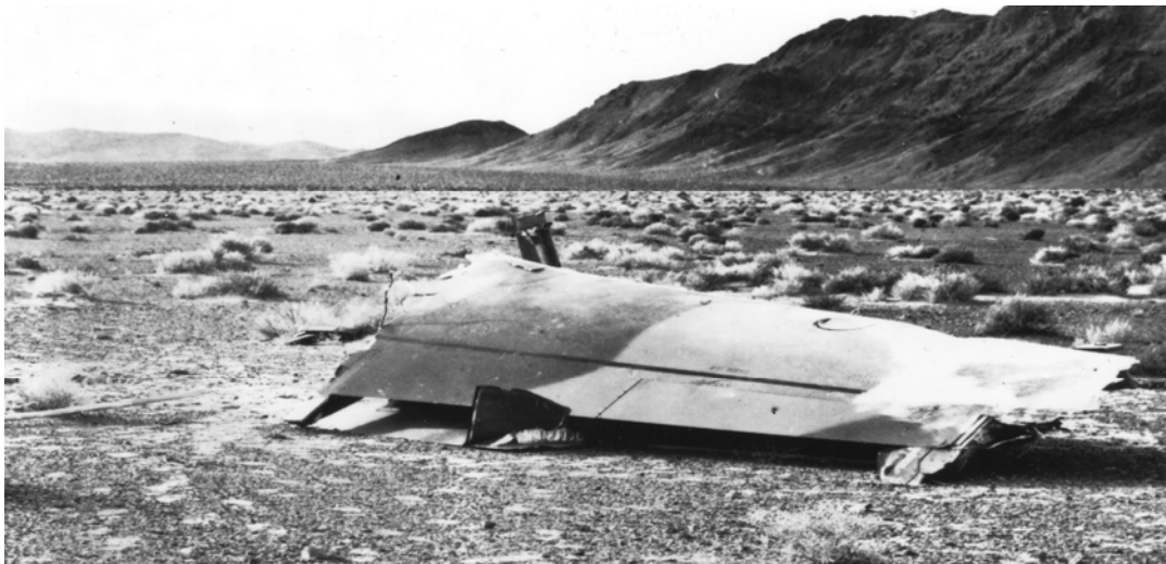
Figure 3-10. F-111A Wing Failure Dec 1969
