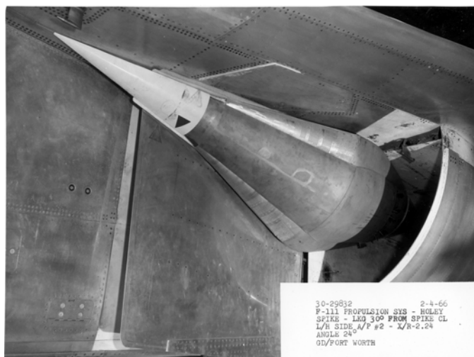
Figure A7-1. Original F-111A Inlet. Note Flat Splitter Plate and Wedge-shaped Ducts Next to Fuselage and Wing that Capture Boundary Layer and Duct it Aft.
